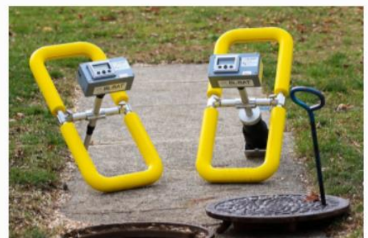
Undated photo of the SL-RAT equipment used to detect sewer blockages using sound waves | Photo courtesy City of Ivins Public Works, St. George News
