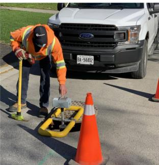
The SL-RAT is an acoustic pipe inspector that uses sound to determine if there is clear flow through each section of sewer pipe, or if there are obstructions that need to be dealt with.
