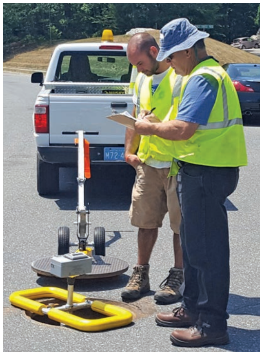
The SL-RAT provides a fast, first-pass screening of collections systems.
