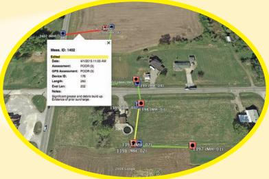
In the field, operators can use the SL-DOG mobile app to add notes to each measurement while conducting tests. Notes such as segment ID or basin ID can be meaningful when referencing the data at a later point. After testing is complete, users upload the assessment scores to the web portal. The comprehensive list of all measurements historically uploaded to the portal can generate useful reports and visualizations.
