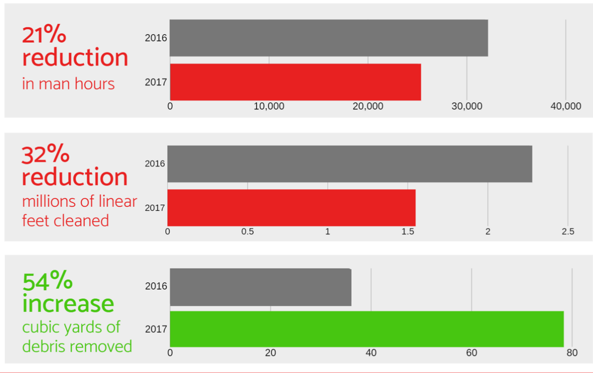
Figure 2. In the first year of implementation (2017), LRWRA was able to drastically reduce time and resources spent cleaning, while significantly improving the amount of debris removed from the system, showing that utilizing acoustic technology as a preliminary tool helped to save time, water and money later in the workflow.
