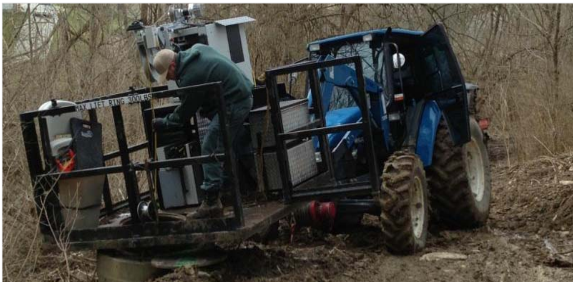
Figure 1-1. Custom Off-road CCTV Camera Tractor (Courtesy: MSDGC).
