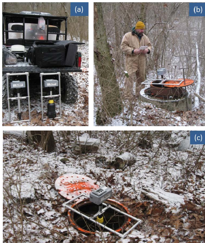
Figure 1-3. SL-RAT Deployment at EPA Project Site: (a) TX and RX Units in Transport Mode, (b) RX Unit Operational Mode Deployment, (c) TX Unit Operational Mode Deployment.
