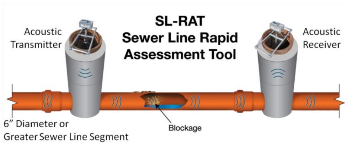
Figure 1. Operation of the Acoustic Inspection System
