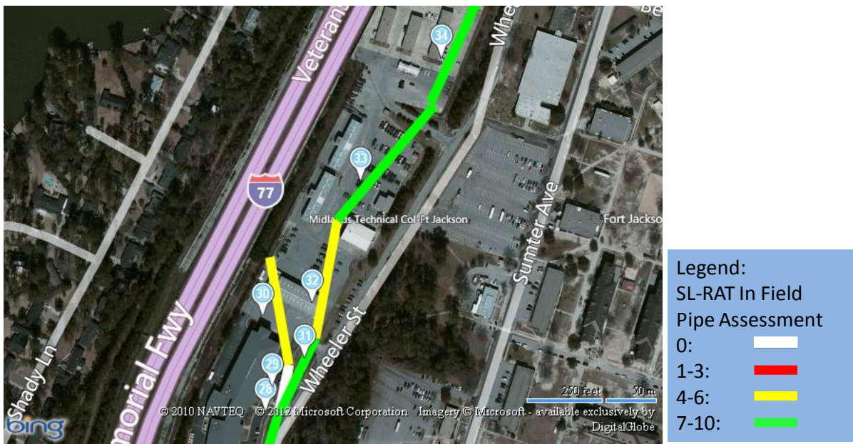
Figure 3. SL-RAT acoustic classification results overlaid on GIS map.
