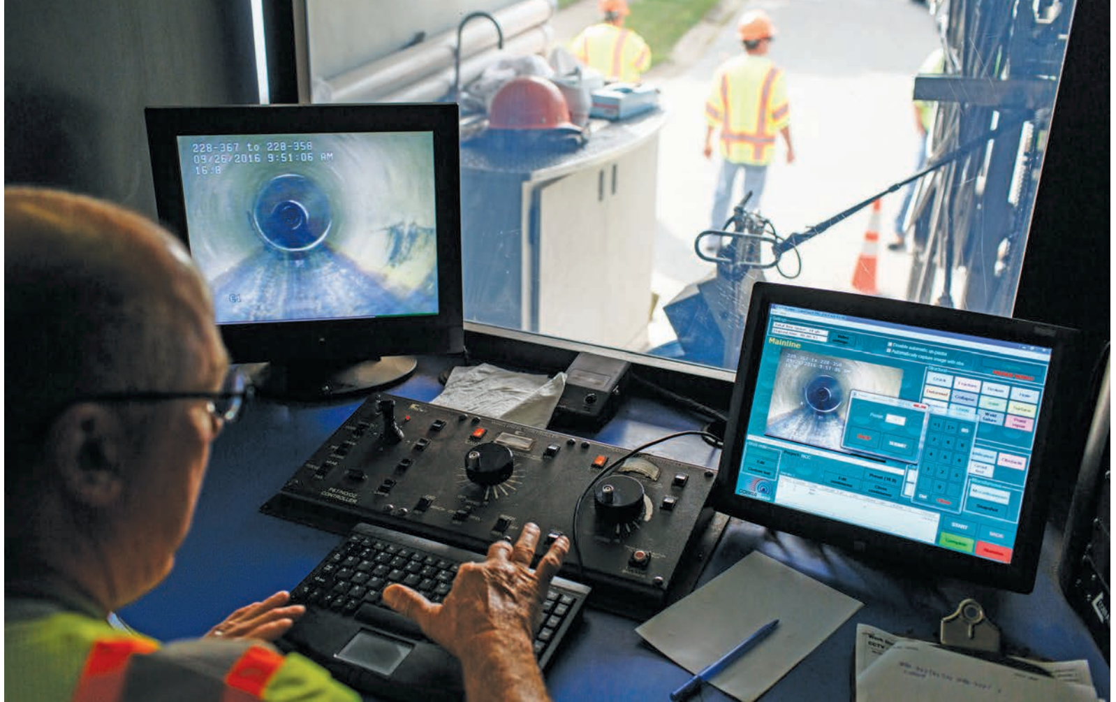
Camera operator Gary Guillotte runs an inspection from the control room of the CUES-equipped CCTV van using Cobra Touch software.
