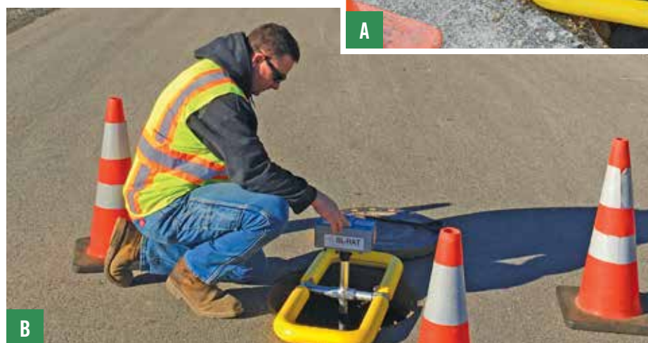
A: Two inspection specialists with the system. B: The SL-RAT being lowered into a manhole.
